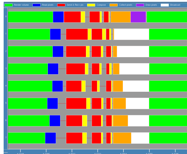
Figure 1: Typical run of the binary-swap volume renderer with 8 nodes (512x512 resolution).
